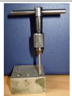
Photo Peter Downes A tapping block drilled for several different sizes of tap.
