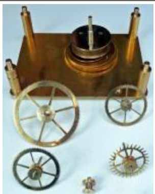
Photo Derek Tulley Finished gears and escapement parts.
