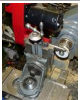
Photo Derek Tulley Gear Cutting on the Lathe.
