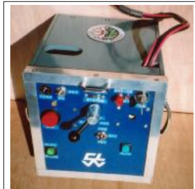
Photo John Brotherton The assembled Power Box showing the controls.
