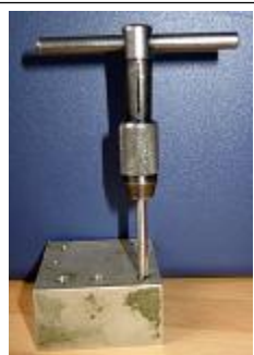
Photo Peter Downes A tapping block drilled for several different sizes of tap.
