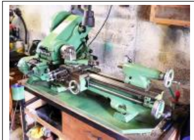
A typical model engineers lathe, the Myford 7. Note the lack of provision for using any coolant.
